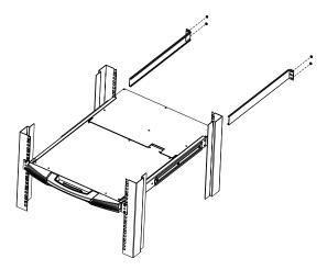
4. After the L brackets have been secured, tighten the front bracket screws.
